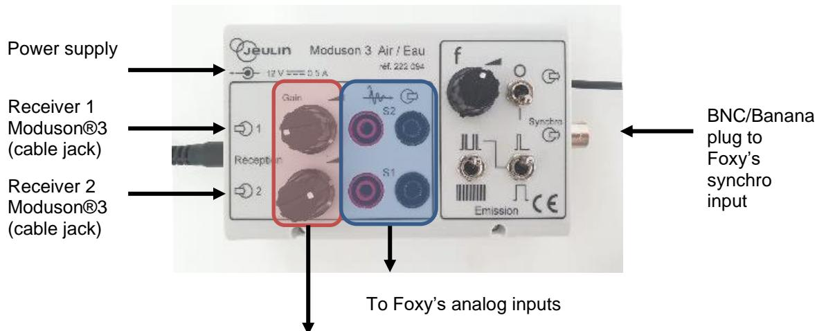
The transducers of the new versions of Moduson® allow a use in the fluids and in the air.
