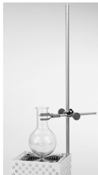
Fixation of a round bottomed-flask using a rod for LAB 2 and LAB3 electric burners. (ref. 703 087).
