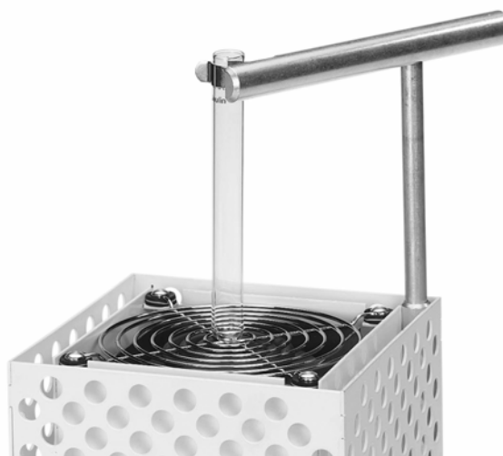
Fixation of a test tube using a glass support (ref. 703 522)
