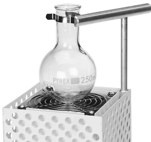
Round-bottomed flask retention with the support for glassware (ref. 703 522)
