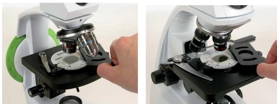
Turn the graduated disc: the central mineral should stay in the middle of the field of view. If necessary, move the device on the stage, turn again the graduated disc to get the minerals centered in the field of view. Try again with an higher magnification: the polarizing stage is now centered.
