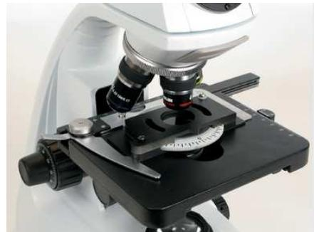
Select the lowest magnification. Focus the device turning the graduated disc and try to keep the minerals in the field of view.
