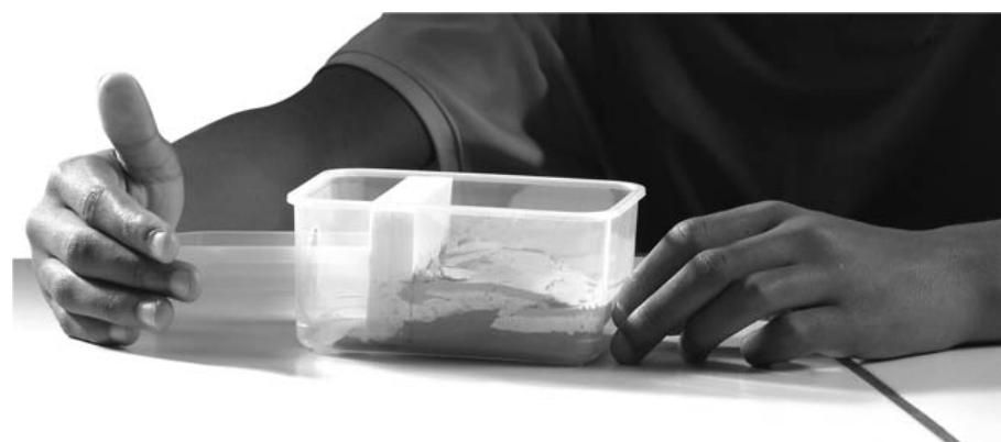
With the layers of material in place, in one hand hold the end of the tank containing the layers to be compressed.
