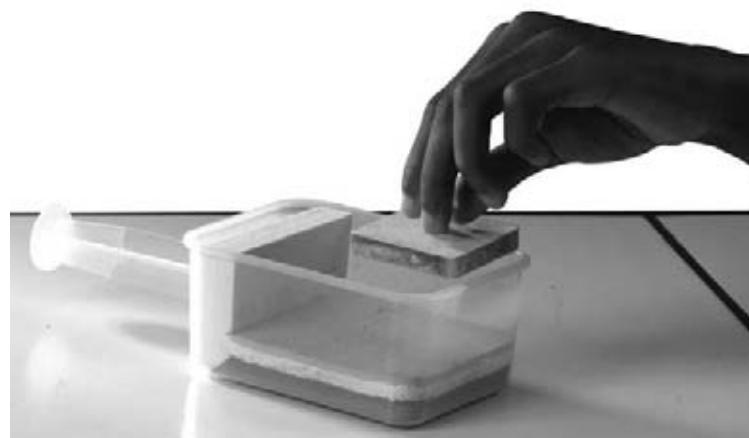
Increase the working distance by withdrawing the pushing device on the piston side.
