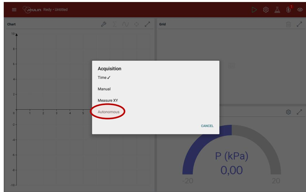
In the tab Configuration, select the acquisition duration using the drop-down menu:
