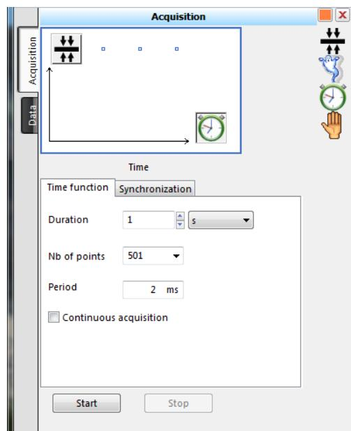
Hence, the user can, if he likes, modify the acquisition duration and/or the number of points. Once the configurations are done, start the acquisition by pressing on the button « Start » (see above).
