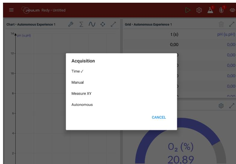
In the tab Configuration, select the acquisition duration using the drop-down menu:
