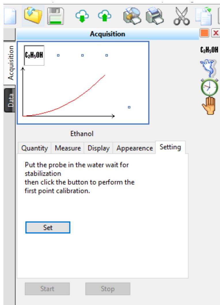
Follow the indicated protocol by placing the probe in the water and click set to validate the first measurement point of the calibration.
