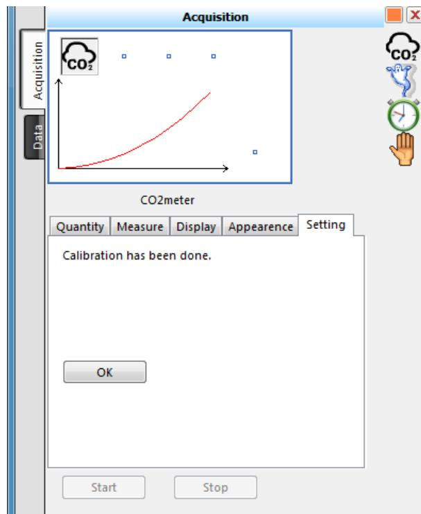
You can check in the Measurement tab that the measured value is now 0.04%.
