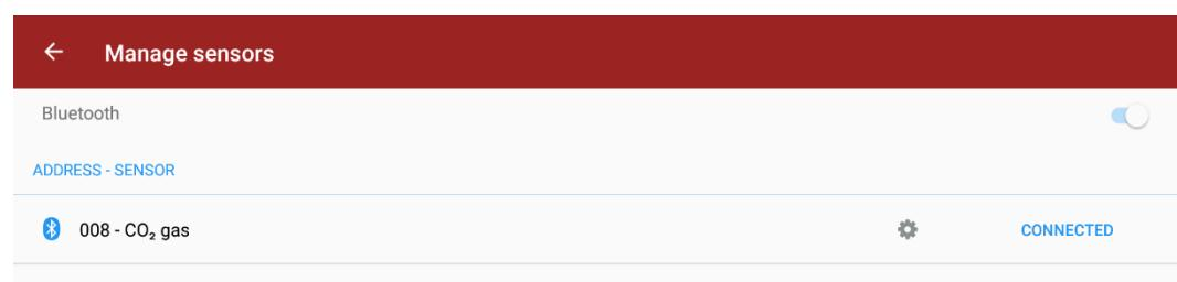
Note the apparition of the Bluetooth logo
