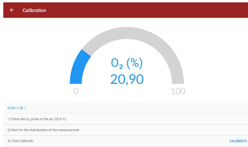
You can check on the screen that the measured value is now 20.9%, the oxygen content of the air.
