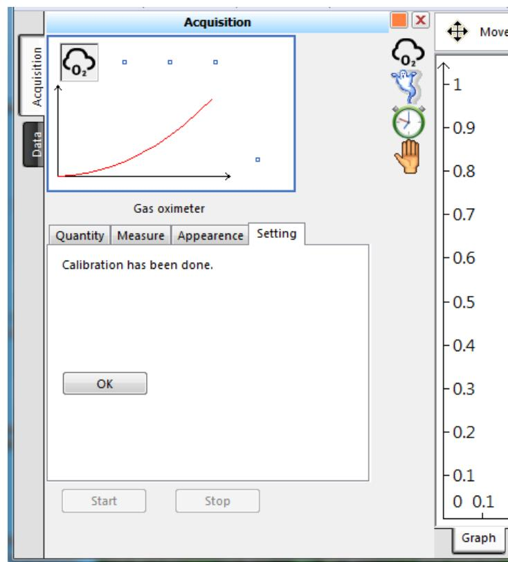
You can check in the Measurement tab that the measured value is now 20.9%, oxygen content in air.
