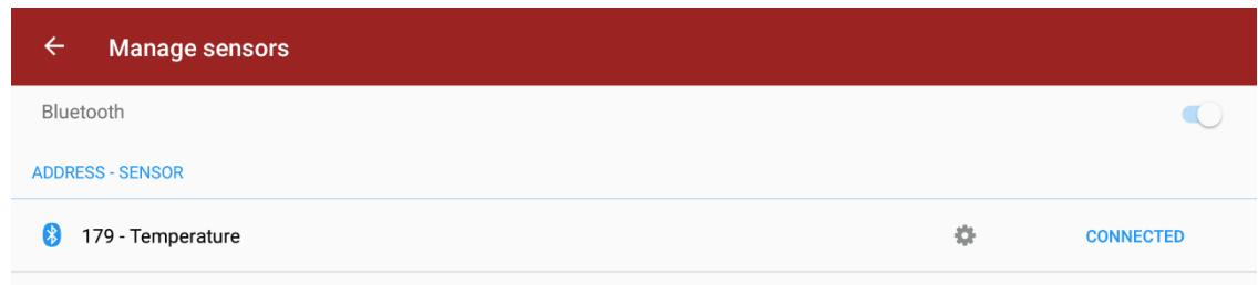
Note the apparition of the Bluetooth logo
