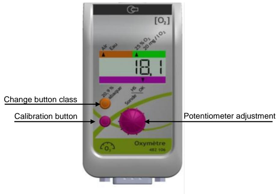
This sensor operates with a console, in standalone mode (without computer) or in connected mode (with computer) after being connected to the console.
