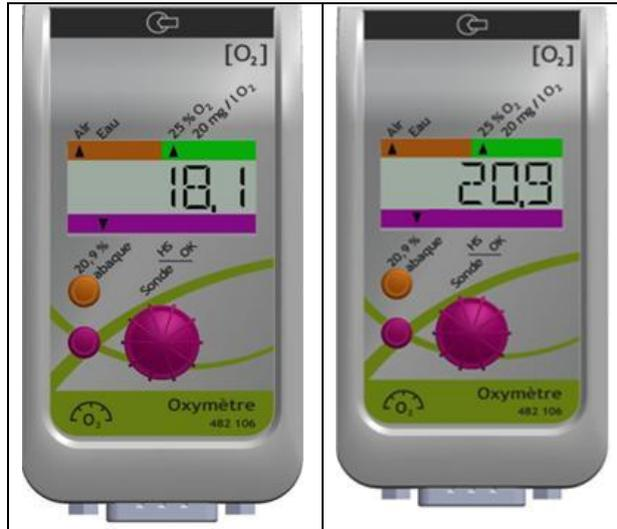
If you are making a measurement in Air, simply fix the value to 20.9 % O<sub>2</sub>. If the displayed value is too far from 20.9 %, make a long press on the calibration button. A flashing arrow appears above the 20.9% reading.
