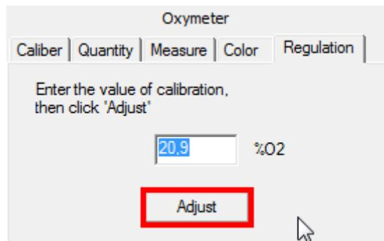
The « Adjust » button is surrounded with a red edging which indicates that the system is verifying the data provided by the probe.
