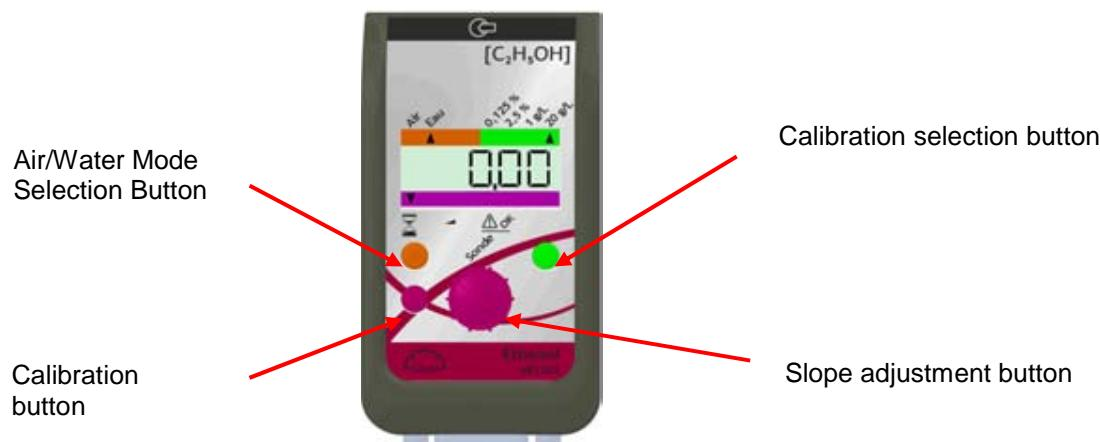
Select the required experiment medium (air or water) by pressing the orange button.
