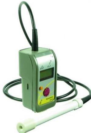
This sensor, with an integral or remote microphone, allows acquiring an audible signal via both microphones and measuring its intensity in decibels using the integral microphone. With a remote microphone, the audible signal is measured exclusively in UA (arbitrary unit). In this case the function dB(A) is deactivated and the function mode button is inactive.
