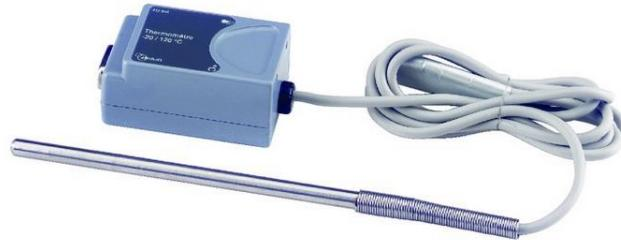
This sensor enables measurement of temperature from -20 to 120°C with the VTT system. The probe used is a 316L stainless steel probe (pharmaceutical quality) of Pt1000 type. This sensor is used with the VTT® and Primo® interfaces.
