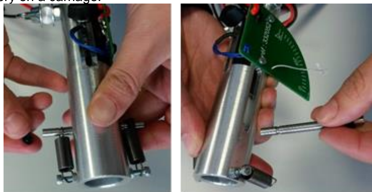
Remove the two rubber end pieces from the pin connecting the two springs. Slide the pin outside the launcher
