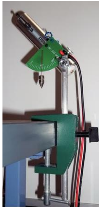
Fig. 2- Ballistic launcher fixed to a bench with its bench mounting
