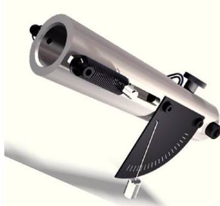
Fig. 12- 3D image of the ballistic launcher
