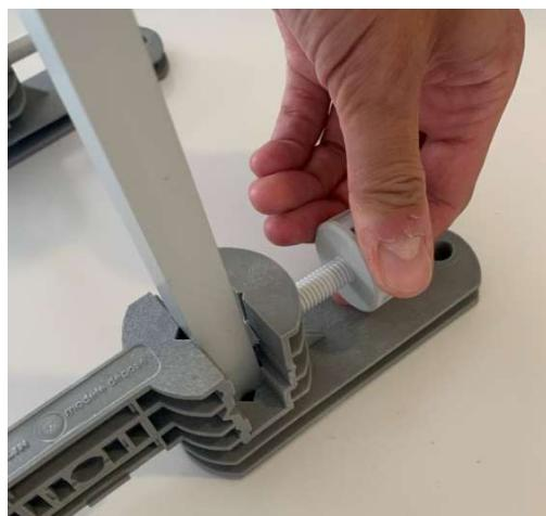
**Step 4:** Position the 2 Polynux nuts in this way on each foot respecting the directions of insertion indicated by the arrows and allowing a height of around 15 cm between the upper part of the foot and the nut
