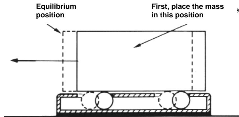
Let  $\alpha$  the angle of the rail relative to the horizontal plane (as read on the graduated dial),  $F$  the mass hung on the wire (the hook mass shall be taken into account as required) and  $P$  the mass of the parallelepiped (weighed beforehand).
