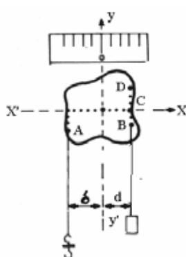
Demonstrate that if force  $\vec{F}_B$  retains the same intensity and the same direction, then movement of the pin around the axis of the force (at C or D on the above diagram) does not modify the equilibrium of the body.
