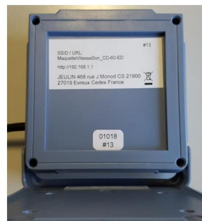
Step 3: From your computing device, select the network that has the same name as the SSID of your apparatus. You can connect up to 4 computing devices to each apparatus simultaneously.
