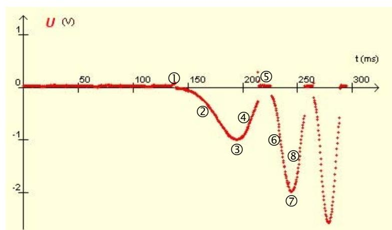
**Remark:** the amplitude of the voltage and of the period varies on account of an increasing speed of rotation
