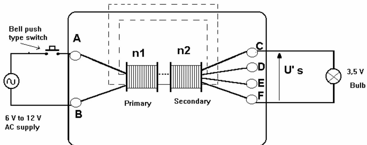
Without a core, the coil has low resistance, and the current is then large: the coil heats and the protective varnish can be destroyed if the current is maintained (particularly at 12 V). To avoid this problem it is recommended that you put a push type switch in the primary circuit.
