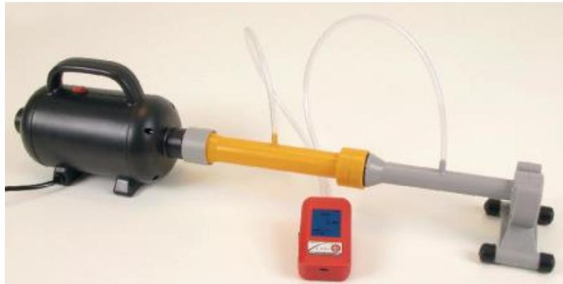
This device allows highlighting Bernoulli's principle, more precisely its specific case : the Venturi effect.
