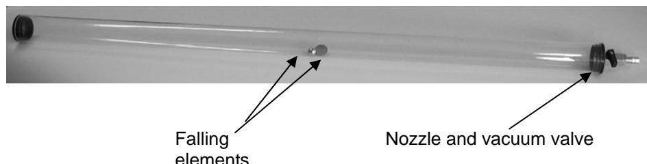
Plastic tube equipped with 2 nozzles and a vacuum valve, containing 2 falling elements: a steel ball and a paper washer.
