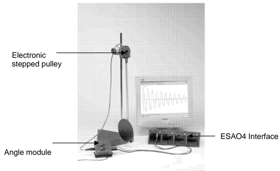
Example of use in Ex.A.O with an ESAO 4 interface, an electronic stepped pulley P/N: 453109 (optional accessory not supplied) and the angle module P/N: 453110 (optional accessory not supplied).
