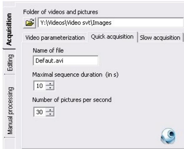
Start the pendulum then start recording by clicking on the webcam icon.
