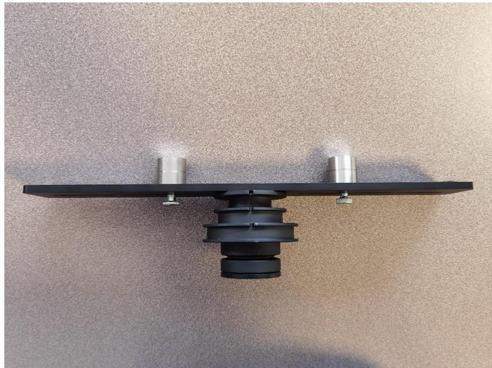
4. **Return pulley on the support:** Connected to the mass, this pulley plays a key role in triggering the rotation when the mass is released.
