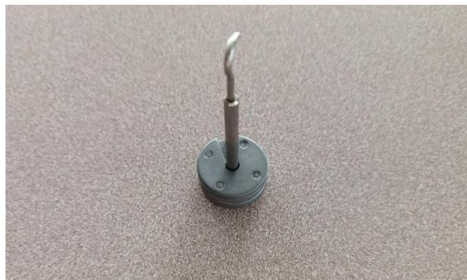
6. **Cylindrical masses:** These additional masses can be fixed on the main axis for various experiments, with wing screws.
